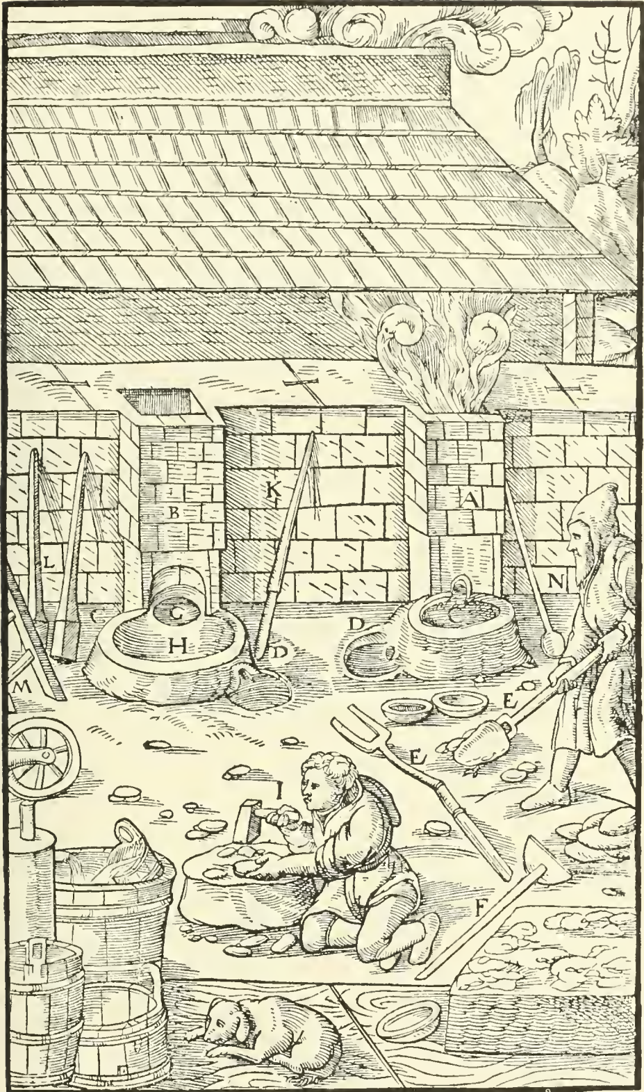
A, B—Two furnaces. C—FOREHEARTH. D—DIPPING-POTS. THE MASTER STANDS AT THE ONE FURNACE AND DRAWS AWAY THE SLAGS WITH AN IRON FORK. E—IRON FORK. F—WOODEN HOE WITH WHICH THE CAKES OF MELTED PYRITES ARE DRAWN OUT. G—THE FOREHEARTH CRUCIBLE: ONE-HALF INSIDE IS TO BE SEEN OPEN IN THE OTHER FURNACE. H—THE HALF OUTSIDE THE FURNACE. I—THE ASSISTANT PREPARES THE FOREHEARTH, WHICH IS SEPARATED FROM THE FURNACE THAT IT MAY BE SEEN. K—BAR. L—WOODEN RAMMER. M—LADDER. N—LADLE.
